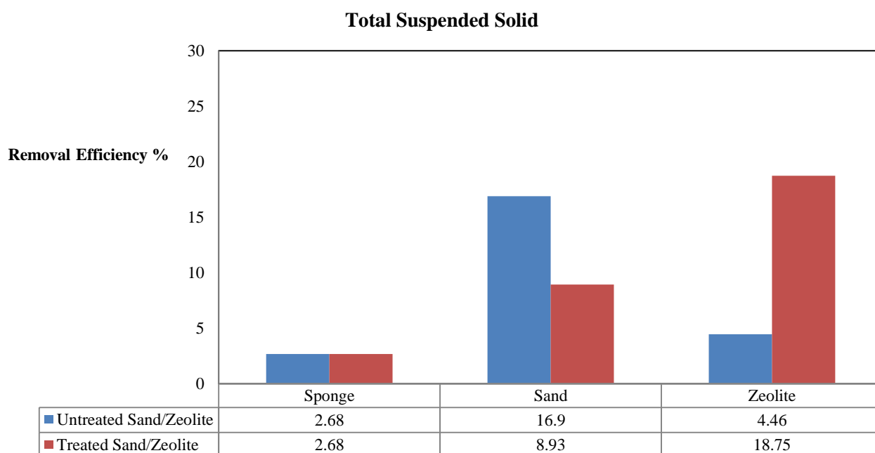
Fig. 5: Removal efficiency of total suspended solid (TSS) on untreated and treated filter media
